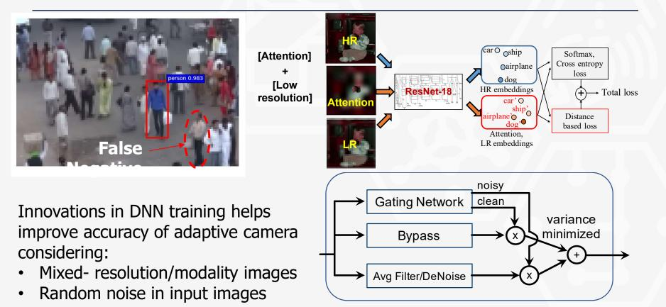
Noise-robust design with mixture of pre-processing engines
