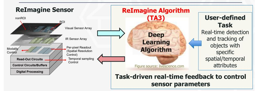
A camera that autonomously controls sensor parameters to increase information content in the picture or video by embedding deep learning algorithms in the processing layer.
