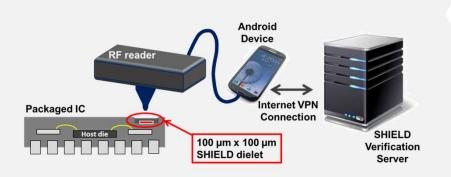
The SHIELD ID chip is referred to as a "dielet" because it is only 100 µm square, smaller than a grain of fine sand. It can be authenticated wirelessly via an RF reader communicating securely over the internet with a remote SHIELD Verification Server, providing a hardware root-of-trust, thus guaranteeing the authenticity of the host IC by making counterfeiting very difficult and prohibitively expensive.
