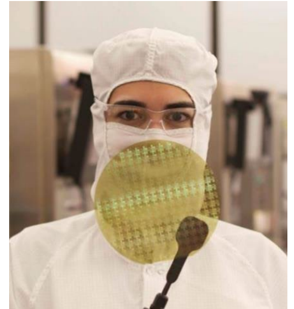
6" SiC wafer processed in Si CMOS foundry
