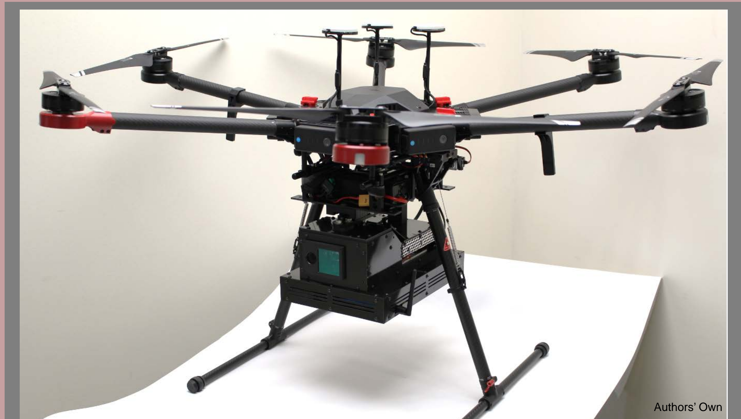
Phase 2 LIDAR payload integrated with a multirotor platform
