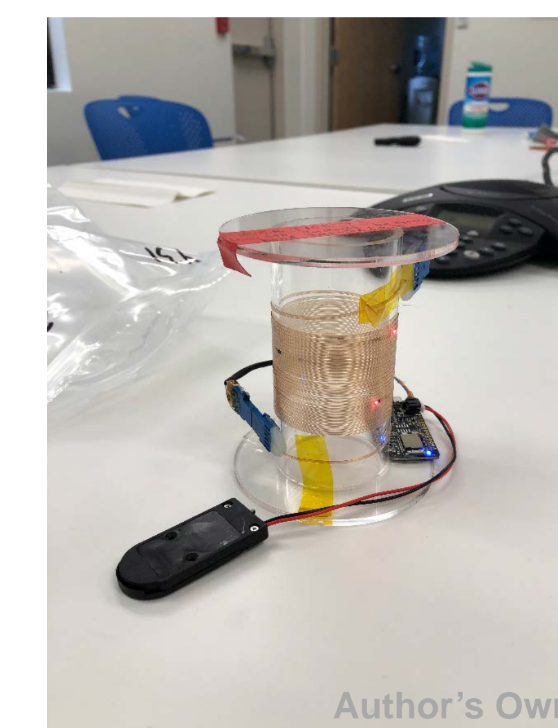
Spool of 5-meter fiber with embedded sensors and illuminated LEDs
