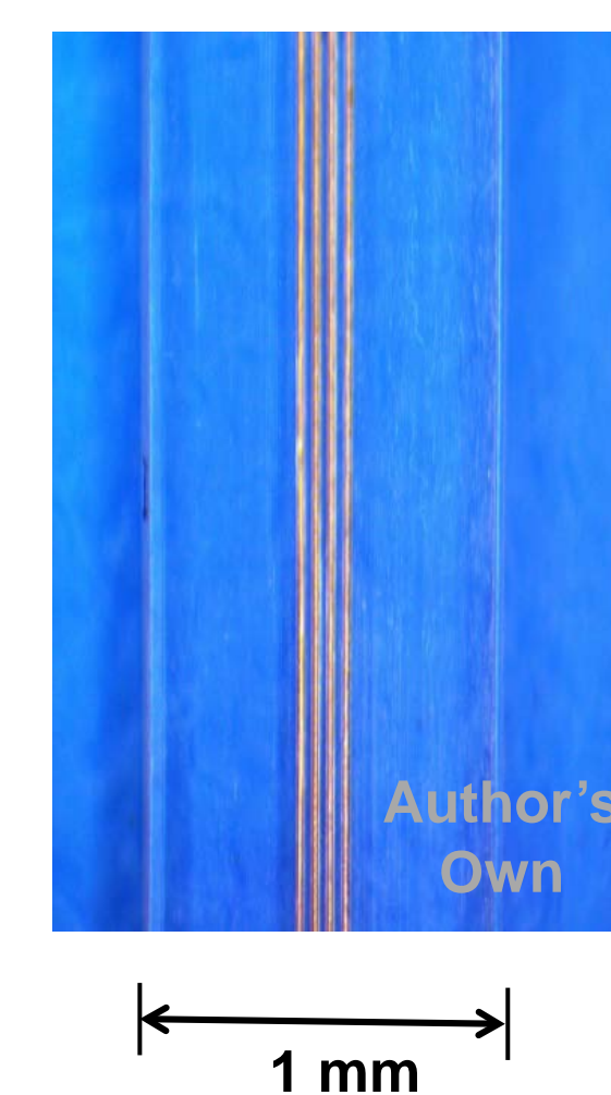
Four copper wires drawn in parallel inside a polycarbonate fiber
