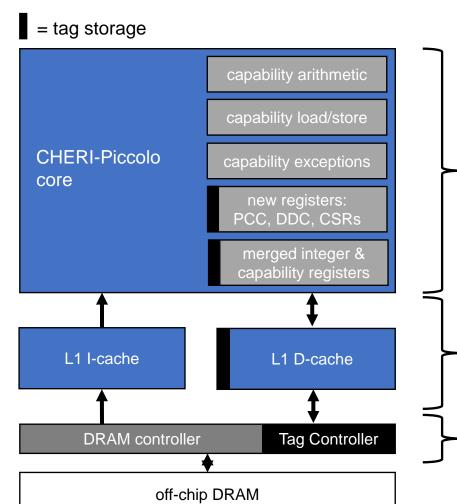
Changes to the Piccolo core (RISC-V 3-stage pipeline): capability arithmetic
